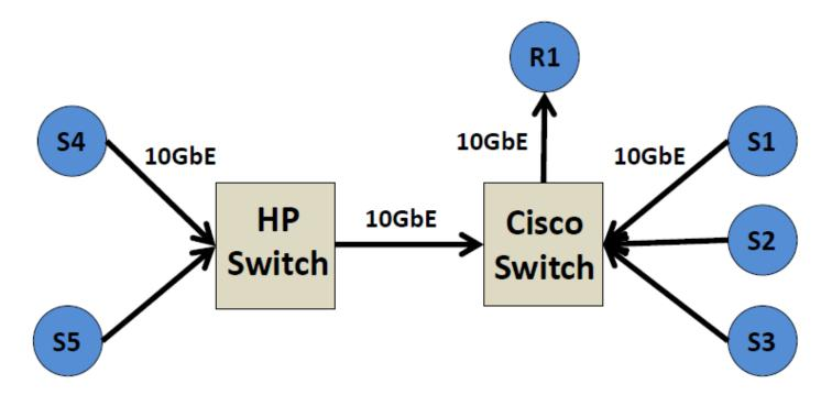
Each of five senders S1, S2, S3, S4, S5 send one flow to receiver R1. The two flows from S4, S5 are called cross-switch flows. The three flows from S1, S3, S3 are called intra-switch flows.
